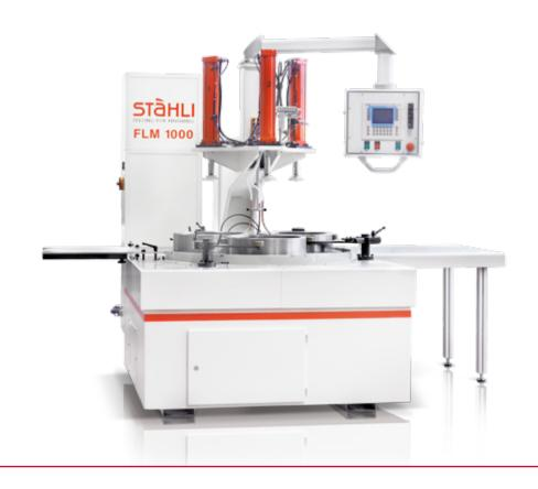
The 1-wheel flat lapping and polishing machines of the FLM series with wheel diameters from 500 to 4000 mm are perfectly optimized for production output.
