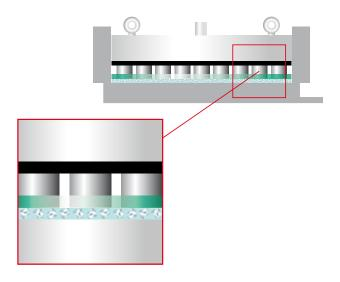
Lapping process with vehicle and loose abrasive.  $(\mathrm{SiC,\,AI_2O_3,\,B_4C})$
